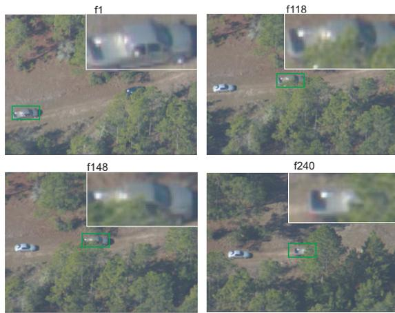
Fig. 3. Tracking results for Egtest05. The proposed tracker can deal with occlusions in the sequence.
