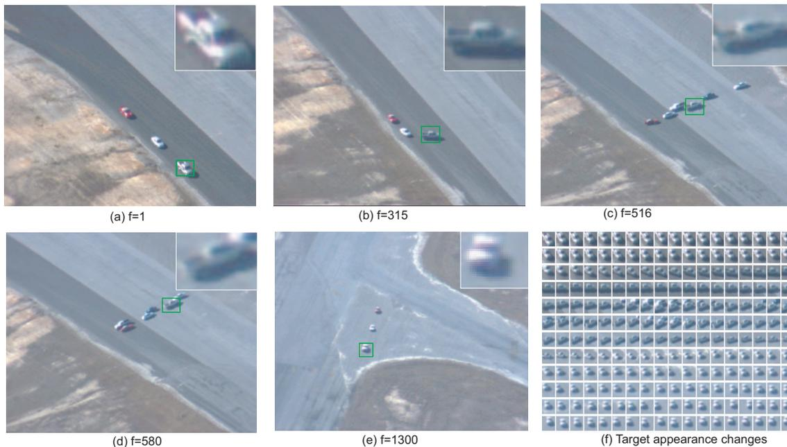
Fig. 6. Tracking results for the EgTest02 sequence using the proposed tracker. Cars similar to the target are threats to robust tracking in the sequence. Both the target and the background have large variations in appearance.
