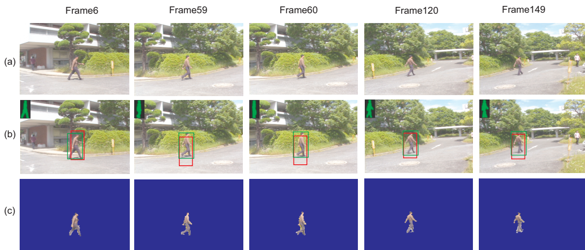
Figure 4: Tracking and segmentation results of the outdoor sequence. (a) Input images; (b) Initial bounding boxes (in red) generated by the tracker, optimal bounding boxes (in green) and gait models (phase) computed by the optimal path searching using DTW; (c) Segmentation results by embedding the shape priors into the Min-Cut algorithm.
