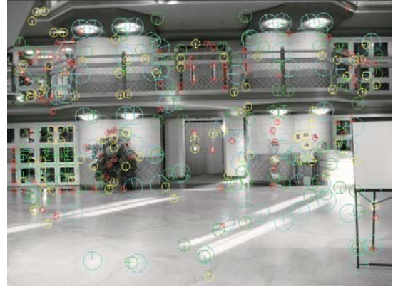
Fig. 2. Interest points detected by Harris-Laplace detector. The centers of the circles are Harris-Laplace interest points. The radiuses of the circles indicate the characteristic scale of interest points.
