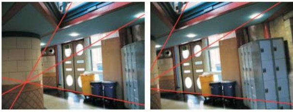
Fig. 6. Left, location retrieved from database (L12 in Fig. 4). Right, image for localization (T2 in Fig. 4). Localization is correct although the angle between them is 20 degrees.
