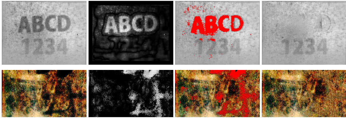
(a) Inner slice including shadow (b) Likelihood of shadow (c) Shadow region mask (d) Inpainted inner layer
