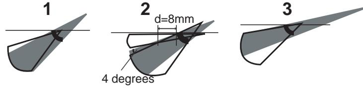
**Fig. 12.** The gray areas indicate the fields of view and the areas closed with solid lines indicate the fields of illumination. For Directions 1 and 3, the field of view indicated by the gray area is covered by the field of illumination indicated by the solid lines. For Direction 2, the area illuminated insufficiently is about 4 degrees. However, if an observed object is close to the endoscope, it can be illuminated.
