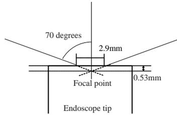
**Fig. 5.** The viewing angle of the endoscopic camera is 140 degrees diagonally. Since the diameter of the lens is 2.9mm, we assumed that the focal point of the camera was 0.53mm inside the lens front.
