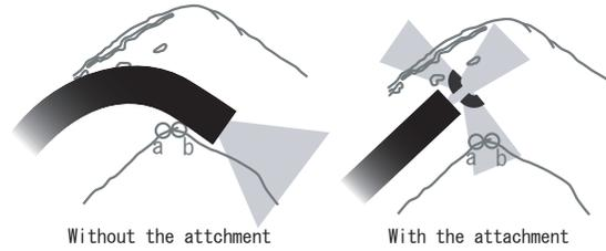
**Fig. 19.** The attachment enables the observation of the inner side of a bending section without complicated manipulations of the endoscope.
