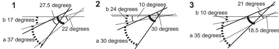
**Fig. 11.** The measured results of the backward field of illumination in three directions in Fig. 8: the solid lines indicate the light by the near one and the dashed lines indicate the other of two light sources. The thick curved lines indicate the position of the mirror. The angle  $a$  of the illuminated area and the angle  $b$  between the horizontal line and the illuminated area were measured.
