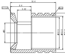
**Fig. 3.** Cross-sectional view of the experimental attachment.
