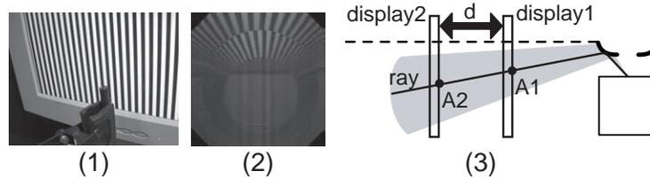
**Fig. 7.** (1) The field of view is measured by using structured light on a flat display. (2) An example of the camera image of the structured light. (3) the direction of a viewing ray is computed by projective structured light patterns from the display at two positions, for which the relative distance  $d$  was known.
