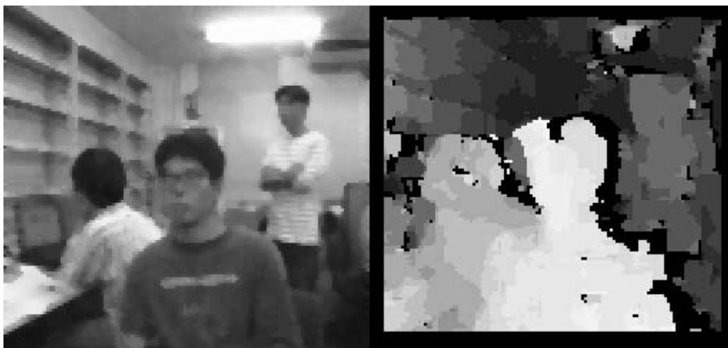
図 1.2: Camera image and dense depthmap
