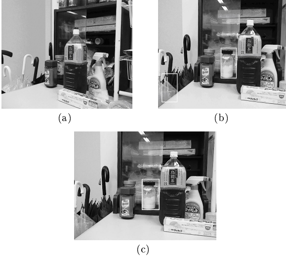
Figure 13 (a) The required object is not found due to occlusion (b) Two objects have been found after the robot moved to the left. The left object is false positive (c) False positive is removed through user interaction.
