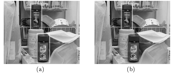
Figure 12 (a) Two objects have been found where the lower one is false positive (creamer) (b) False positive is removed through user interaction.
