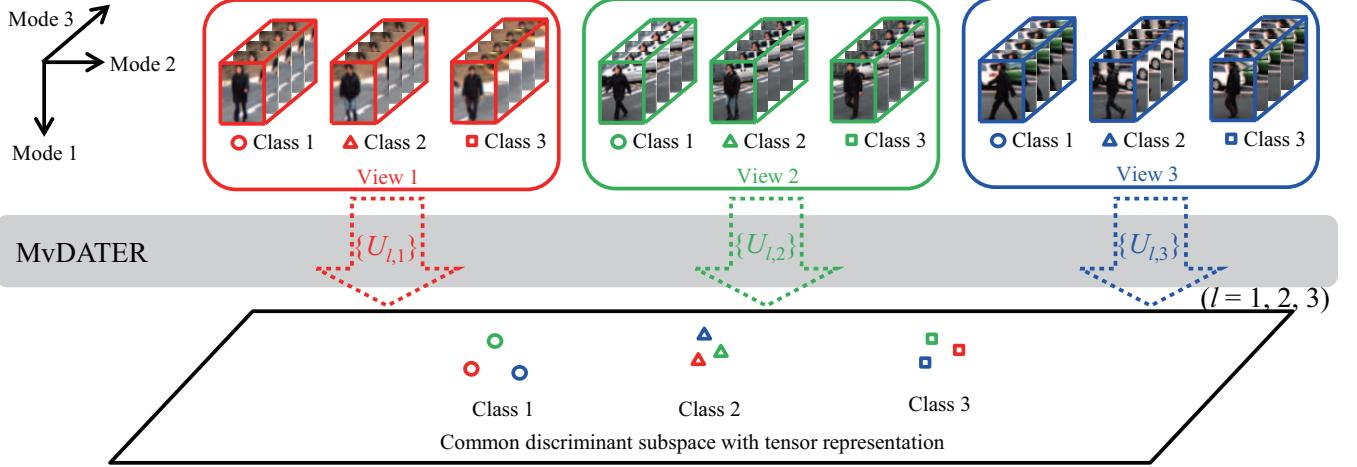
Fig. 1. Overview of MvDATER. In this example, a spatio-temporal image is treated as a third-order tensor and vertical, horizontal, and temporal axes are regarded as mode 1, 2, and 3, respectively. An objective of the MvDATER is to obtain a common discriminative tensor subspace using mode-specific and view-specific projection matrices  $\{U_{l,j}\}$ , where  $l$  and  $j$  are mode and view indices, respectively.
