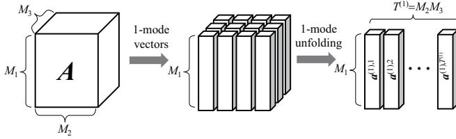
Fig. 2. Illustration of the 1-mode vectors and unfolding.
