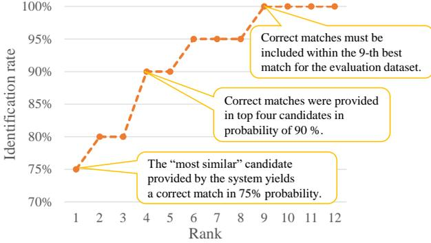
Figure 5: Example of CMC curves, which are utilized for evaluating the identification performance.
