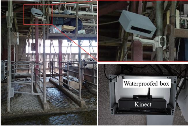
Figure 2: RGB-D image capture system.
