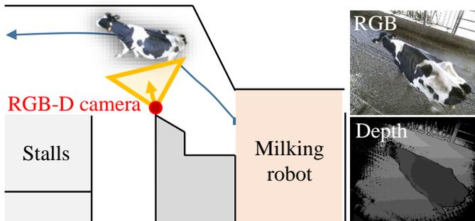
Figure 3: Sensor setting for the experiment.
