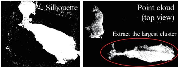
Figure 8: The largest 3D point cluster is extracted for isolating multiple overlapping cows in a silhouette image.
