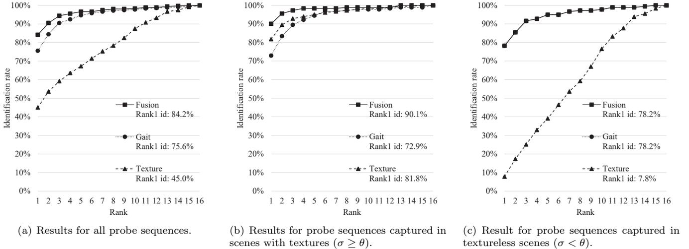
Figure 15: CMC curves of cow identification. The fusion of two identification cues achieves high identification accuracies in every environment. In textureless scenes (night or textureless cows), texture identification gives nearly chance-level results (a rank-1 identification rate of 7.8%). Note that the dissimilarity of the fusion method is equal to the dissimilarity of gait features in (c); thus, the two CMC curves overlap.
