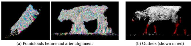
Figure 10: 3D alignment result. (a): Point cloud of each frame combined using different colors. (b): Outliers of the ICP algorithm based on RANSAC-based outlier rejection of a frame.
