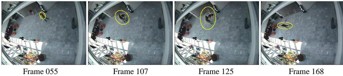
**Fig. 19** Applying the RKM into object tracking. This video is taken from the public database of PETS-ECCV2004, and in this sequence the target person is fighting against another person. The RKM-based tracking system has successfully tracked the target person against the other person.
