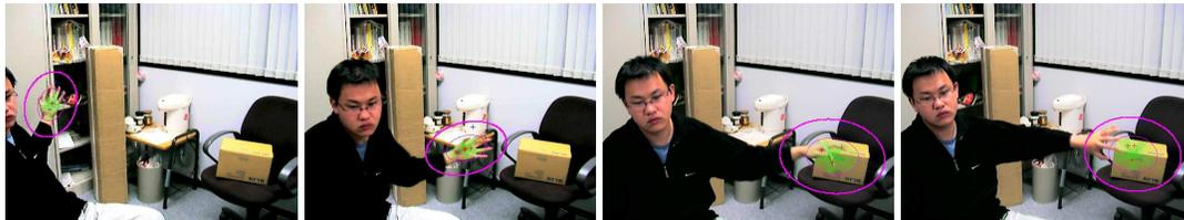
Results of the K-means tracker. The missing target center and similar color of background make it failed since Frame 285.
